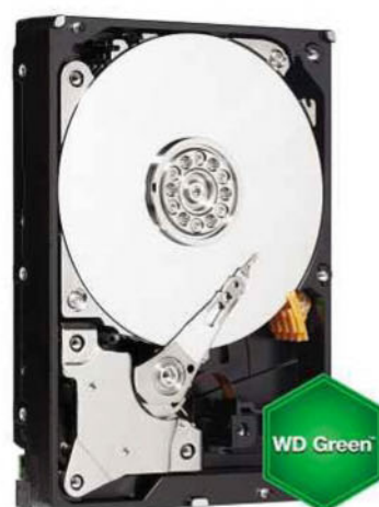
▲ By increasing the areal density, WD can fit in 1.2TB per platter
