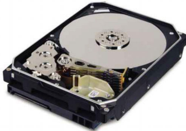
▲ The helium cause less friction, which allows for more platters
