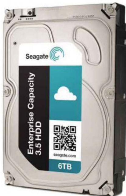
▲ The Seagate 6TB Enterprise drive, with Shingled drive technology
